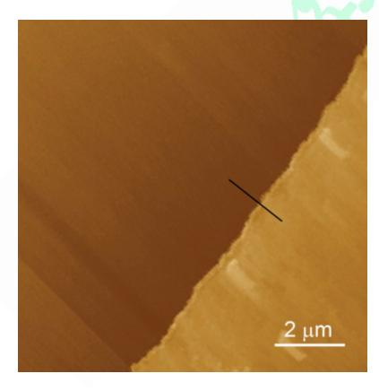
AFM scan of multilayer BN on Cu
